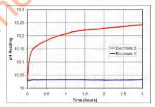
Electrode 1 has been properly cleaned before calibration." Electrode 2 has not been properly cleaned.
