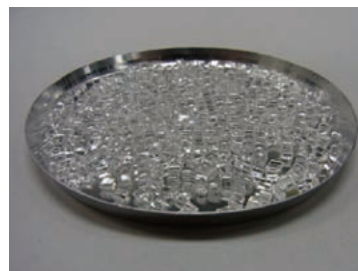
(Before measurement) The sample was spread evenly over the pan.
