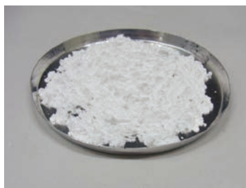
(Before measurement) The corn starch was spread evenly over the pan.
