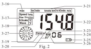
3-16 Max. value indicator 3-22 measurement reading 3-17 Parameter indicator 3-23 Browsing indicator 3-18 Temp. unit 3-24 Number of reading memorized 3-20 Area unit 3-25 Low battery indicator 3-21 Speed & Flow unit 3-26 Memory indicator 3-27 Direction indicator
